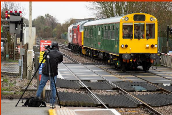
The track inspection saloon and a garishly painted Class 37 arrives at Elmswell. This train allows track and signal engineers a ‘drivers’ eye view of the track.
